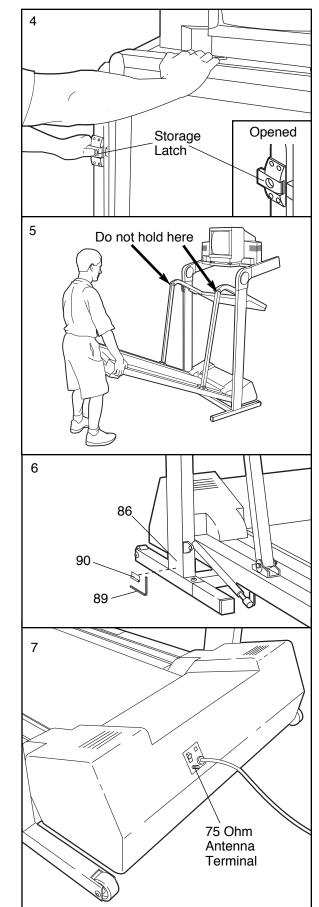
4. Hold the upper end of the treadmill with your right hand as shown. Using your left thumb, slide open the storage latch and hold it open. Pivot the treadmill until the frame is past the storage latch.
